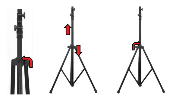
Loosen Knob C by turning it counter clockwise. Extend the inner pipe to the desired height and insert the safety pin through the stopper holes in the inner pipe. Secure and tighten Knob C by turning it clockwise. Repeat this process to set the desired height for inlet pipe as well.
